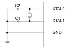
The Oscillator can operate in four different modes, each optimized for a specific frequency range. The operating mode is selected by the fuses CKSEL3:1 as shown in Table 7.
