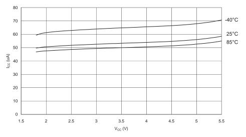
ANALOG COMPARATOR CURRENT vs.  $V_{\rm CC}$
