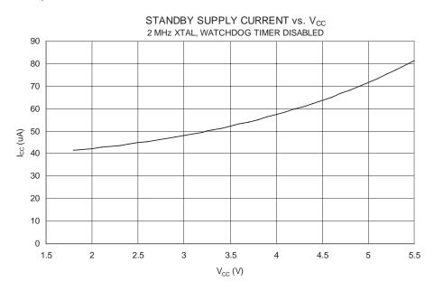
Figure 135. Standby Supply Current vs.  $V_{CC}$  (2 MHz Resonator, Watchdog Timer Disabled)
