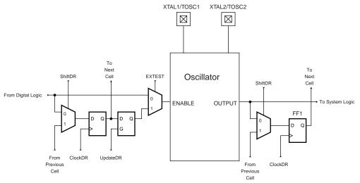
Table 86 summaries the scan registers for the external clock pin XTAL1, oscillators with XTAL1/XTAL2 connections as well as 32 kHz Timer Oscillator.
