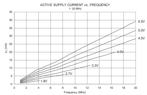
Figure 123. Active Supply Current vs. Frequency (1 - 20 MHz)
