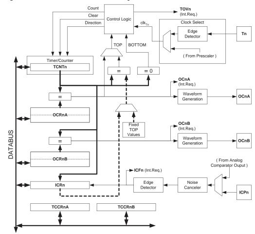
Figure 46. 16-bit Timer/Counter Block Diagram<sup>(1)</sup>
