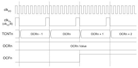
Figure 69 shows the setting of OCF2 and the clearing of TCNT2 in CTC mode.
