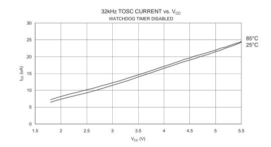
Figure 171. 32 kHz TOSC Current vs.  $V_{CC}$  (Watchdog Timer Disabled)
