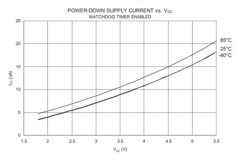
Figure 131. Power-down Supply Current vs. V<sub>CC</sub> (Watchdog Timer Enabled)
