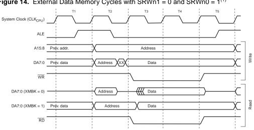
Figure 14. External Data Memory Cycles with SRWn1 = 0 and SRWn0 =  $1^{(1)}$
