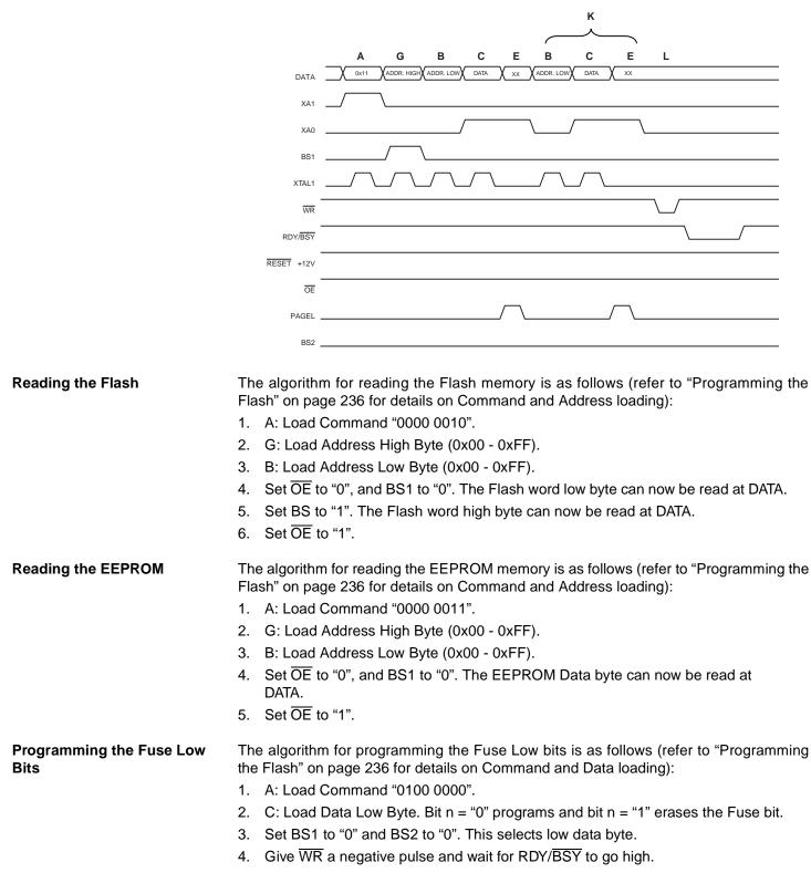
Figure 99. Programming the EEPROM Waveforms
