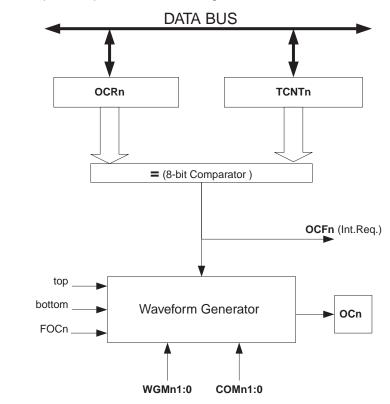
Figure 35. Output Compare Unit, Block Diagram
