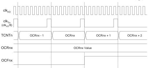
Figure 56. Timer/Counter Timing Diagram, Setting of OCFnx, with Prescaler (f<sub>clk I/O</sub>/8)
