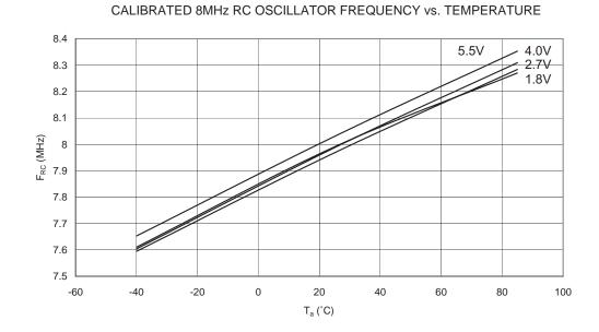
Figure 167. Calibrated 8 MHz RC Oscillator Frequency vs. Temperature
