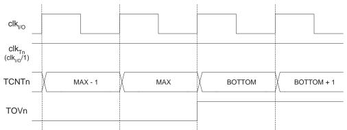
Figure 40. Timer/Counter Timing Diagram, no Prescaling
