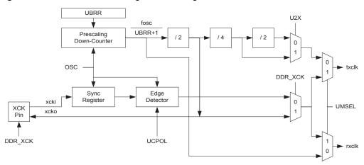
Figure 76. Clock Generation Logic, Block Diagram
