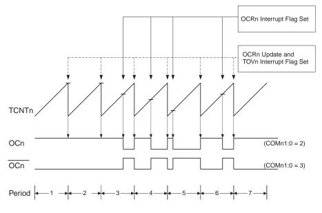
The Timer/Counter Overflow Flag (TOV2) is set each time the counter reaches MAX. If the interrupt is enabled, the interrupt handler routine can be used for updating the compare value.
