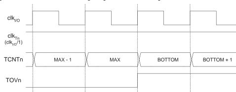
Figure 66. Timer/Counter Timing Diagram, no Prescaling
