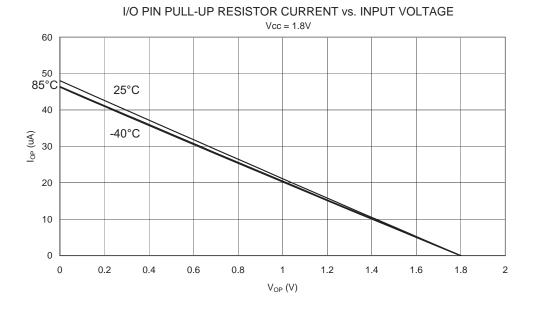
Figure 143. I/O Pin Pull-up Resistor Current vs. Input Voltage (V<sub>CC</sub> = 1.8V)
