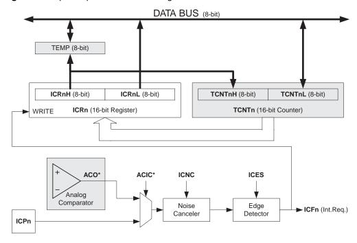
Figure 48. Input Capture Unit Block Diagram<sup>(1)</sup>
