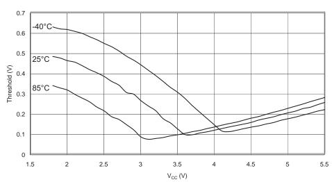
RESET INPUT PIN HYSTERESIS vs. VCC
