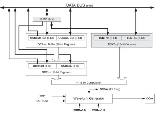
Figure 49. Output Compare Unit, Block Diagram
