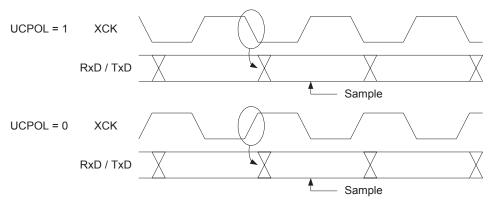
The UCPOL bit UCRSC selects which XCK clock edge is used for data sampling and which is used for data change. As Figure 77 shows, when UCPOL is zero the data will be changed at rising XCK edge and sampled at falling XCK edge. If UCPOL is set, the data will be changed at falling XCK edge and sampled at rising XCK edge.
