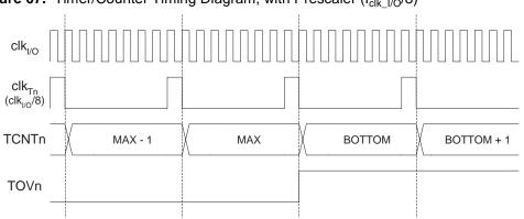
Figure 67. Timer/Counter Timing Diagram, with Prescaler ( $f_{clk\_l/O}/8$ )
