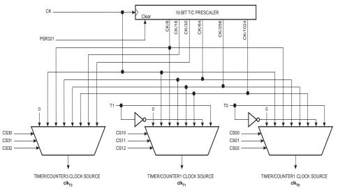
Figure 45. Prescaler for Timer/Counter0, Timer/Counter1, and Timer/Counter3<sup>(1)</sup>
