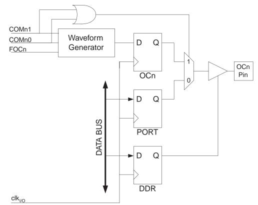
Figure 62. Compare Match Output Unit, Schematic
